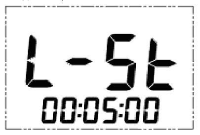
12. Pressing the LEFT ARROW key again displays the current logging stop time (See below). The logging stop time can be changed in menu mode. (See appendix A)
