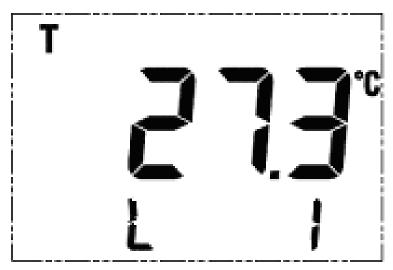
7. "L" will flash when the 367D is logging. Pressing the RIGHT ARROW key will activate and deactivate logging. The number to the right will increase each time a new measurement has been logged.
