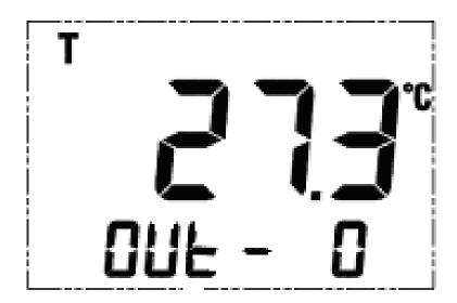
17. Pressing the LEFT ARROW key selects the location to recall and display. Allow 1 second for data retrieval.
