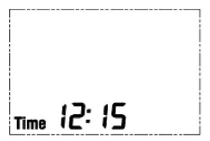
The clock displays in a 24 hour format (hh:mm) and can be set from the menu mode.
