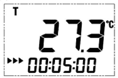
19. Pressing the LEFT ARROW key cycles through the timers. The timers can be set from the menu mode. Pressing the RIGHT ARROW key activates the timer and the arrows on the left side of the timer will begin to scroll. Pressing the RIGHT ARROW key again stops and resets the timer.
